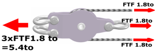
Figure 1: Forces acting on a single sheave pulley
