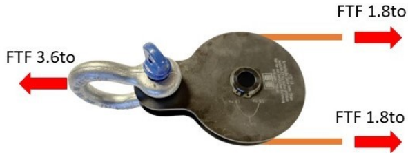
Figure 7: Forces acting on 1-fold pulley
