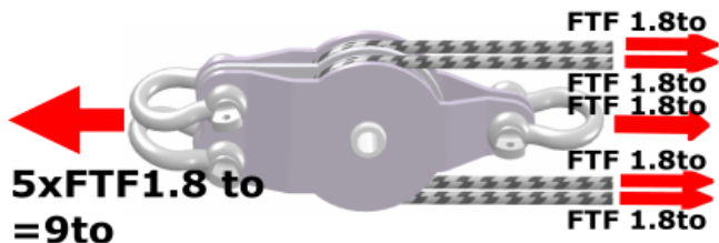
Figure 2: Forces acting on a double sheave pulley
