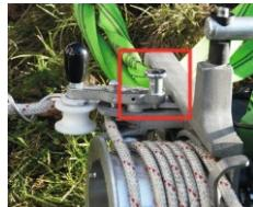
The rope locking mechanism is latched in the half-throttle position. The half-throttle position is released again by drawing on the pulling rope. The half-throttle pin springs back into its original position.
