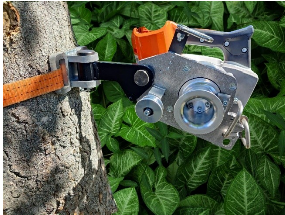
Fig. 9: Mounting the slinging aid
