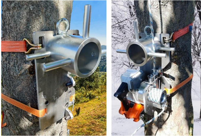
Fig. 6: Mounting the rigging plate
