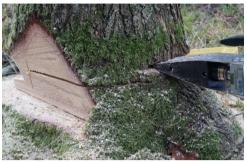
The offset felling cut is obligatory, as it avoids dangerous contact between the Titan 80 Pro and the chainsaw chain.
