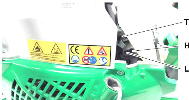
Fig. 20: Carburettor adjusting screws on the motorised handheld device
