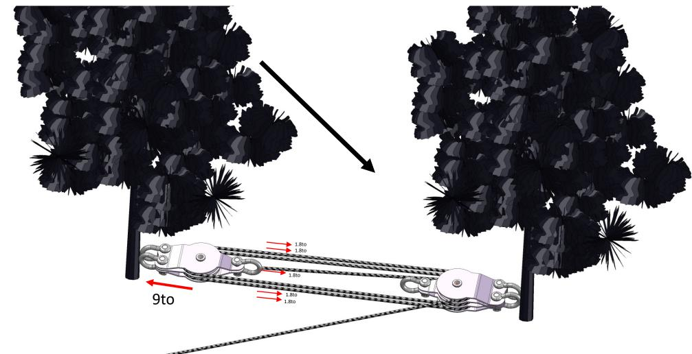
Double pulley as "loose pulley" on which 5 rope strands with 1.8to each act.
