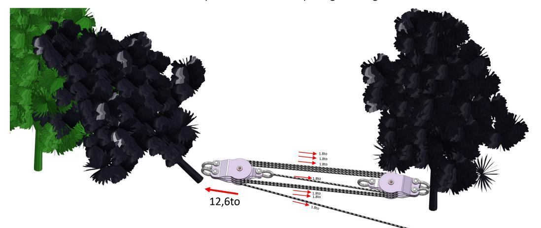
Triple pulley as "loose pulley" on which 7 rope strands with 1.8 to each act.
