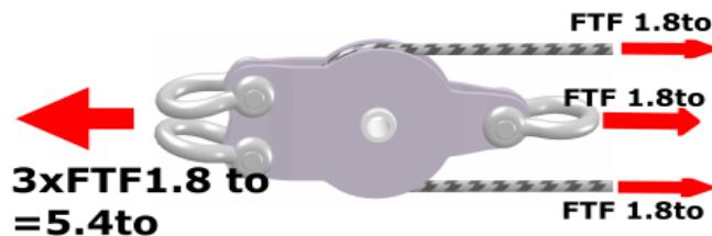
Figure 1: Forces acting on a single sheave pulley
