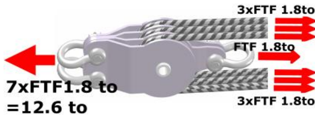
Figure 3: Forces acting on a triple sheave pulley
