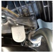
Connect the hydraulic hoses correctly before starting the engine. The pressure line is marked with a "P" on the EDER hydraulic unit. Make sure that the pressure line and the return hose are connected correctly. The hoses and the hydraulic connections on the power unit must be kept clean.
