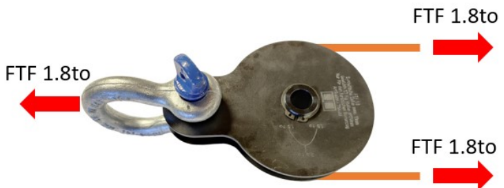
Figure 7: Forces acting on 1-fold pulley
