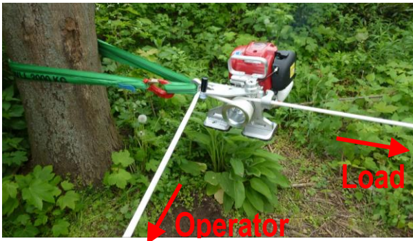
Fig. 19: EDER Powerwinch 500 in working position
