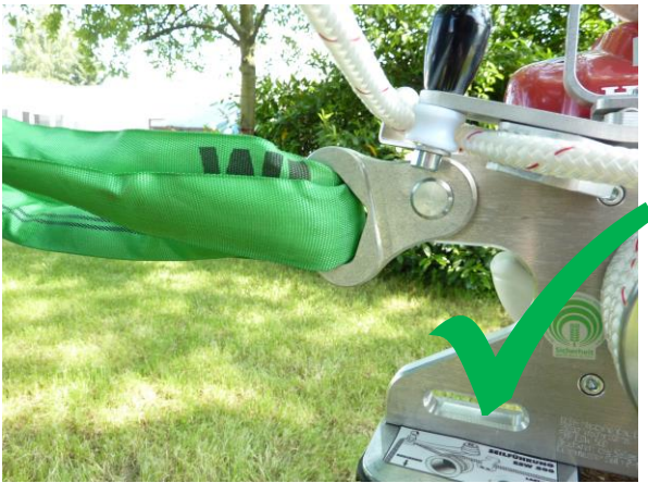
Fig. 22: Correct fastening the EDER Powerwinch 500
