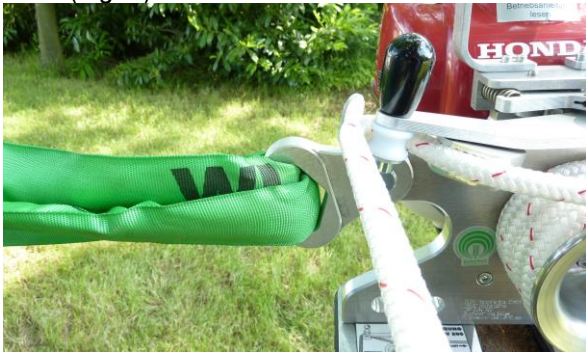
Fig. 20: Guiding the rope through the clamp
