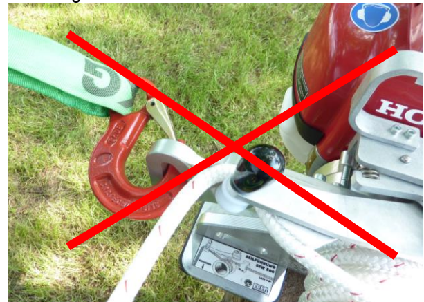
Fig. 21: wrong fastening the EDER Powerwinch 500
