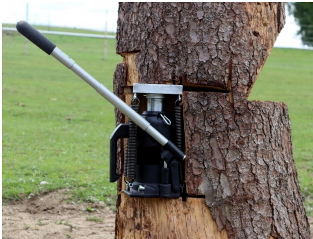
Installed and pre-tensioned lifting cylinder
