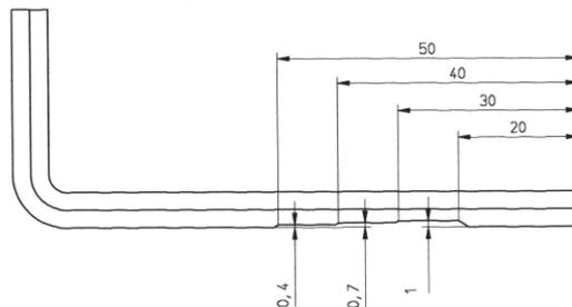
**Fig. 10:** Allen wrench with notches
