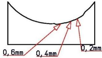
**Fig. 12:** Cutting depths on the knife gauge
