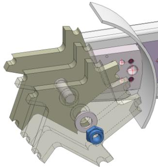
**Fig. 14:** Replacing knives on the groove cutter
