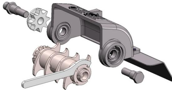
**Fig. 16:** Replacing knives
