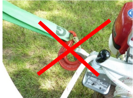
Fig.6: wrong fastening the EDER WINCH 500
