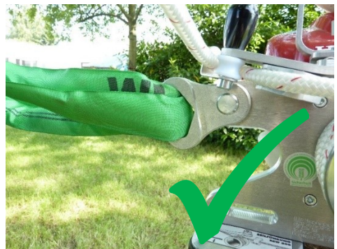
Fig.7: Correct fastening the EDER WINCH 500
