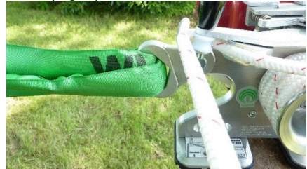
Fig.5: Guiding the rope through the clamp
