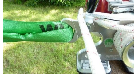
Fig.5: Guiding the rope through the clamp
