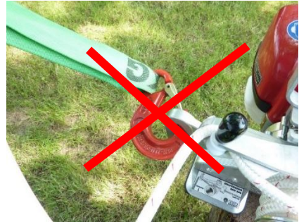
Fig.6: wrong fastening the EDER WINCH 500
